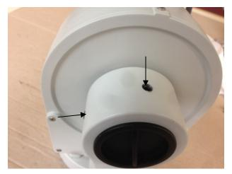
2. Remove 5 screws on the RA ring gear cover and remove the cover to expose the gear/worm.
