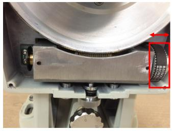
**7. To fix RA worm assembly gap**, fully disengage RA gear switch and rotate the mount head to the side.
