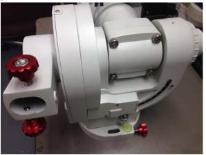
Remove screws that hold Guiding Post panel in place and disconnect two cables (Guiding and RS232).
