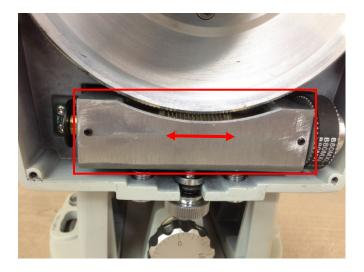
If the brass RA worm, or the worm pulley is moving left and right with turning the RA axle gently, there is a gap between the RA worm and worm bearing. It can be fixed by tightening the RA worm end cap.
