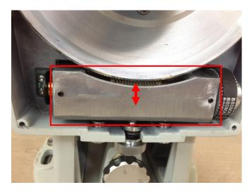
5. If the RA worm assembly is moving left and right with turning the RA axle gently, it means there is a small gap between the RA worm assembly and mounting house. It can be eliminated by tightening the bearing end caps. Refer to Step 7 for how to fix.
