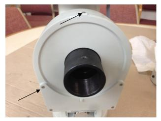
3. Adjust the RA gear switch to make a proper gear meshing as the mount is under operation. There should not have any gap between the worm and gear. Now gently turn the RA axle, check which part is moving. If only the ring gear is moving as indicated, the gear switch is not engaged.
