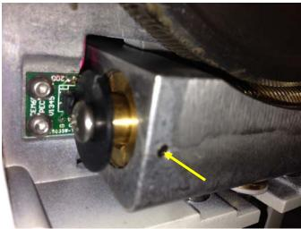
**13.** Using a small screw driver to tighten the worm end cap a little bit. Be careful not to broken the PEC
