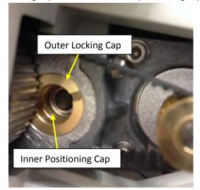
10. Release the outer locking cap a little by turning it counterclockwise (CCW) with a small screw driver. Then turn the inner position cap clockwise (CW) to eliminate any gap. Do not over tighten it. You may check it by engaging the gear switch and rotating the RA axle. Retighten the outer locking cap.
