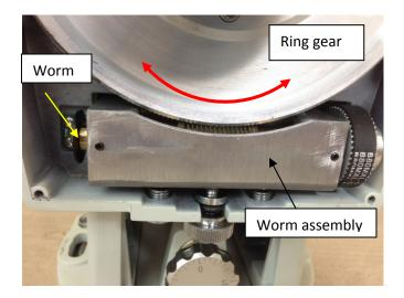
**4.** If the RA worm assembly is moving slightly up and down with quite a bit force applied, the gear is meshed properly. The magnetic force is holding the worm in place.
