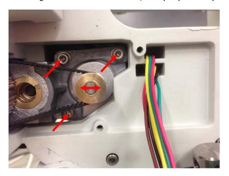
Loosen three hex screws that hold the motor a little bit. Adjust the motor position to adjusting the belt tension. Retighten the hex scews.
