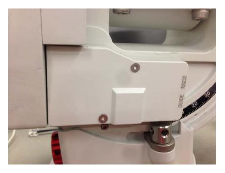
Unscrewing two screws. Remove the RS232/Guide port panel to exposure the R.A. motor.
