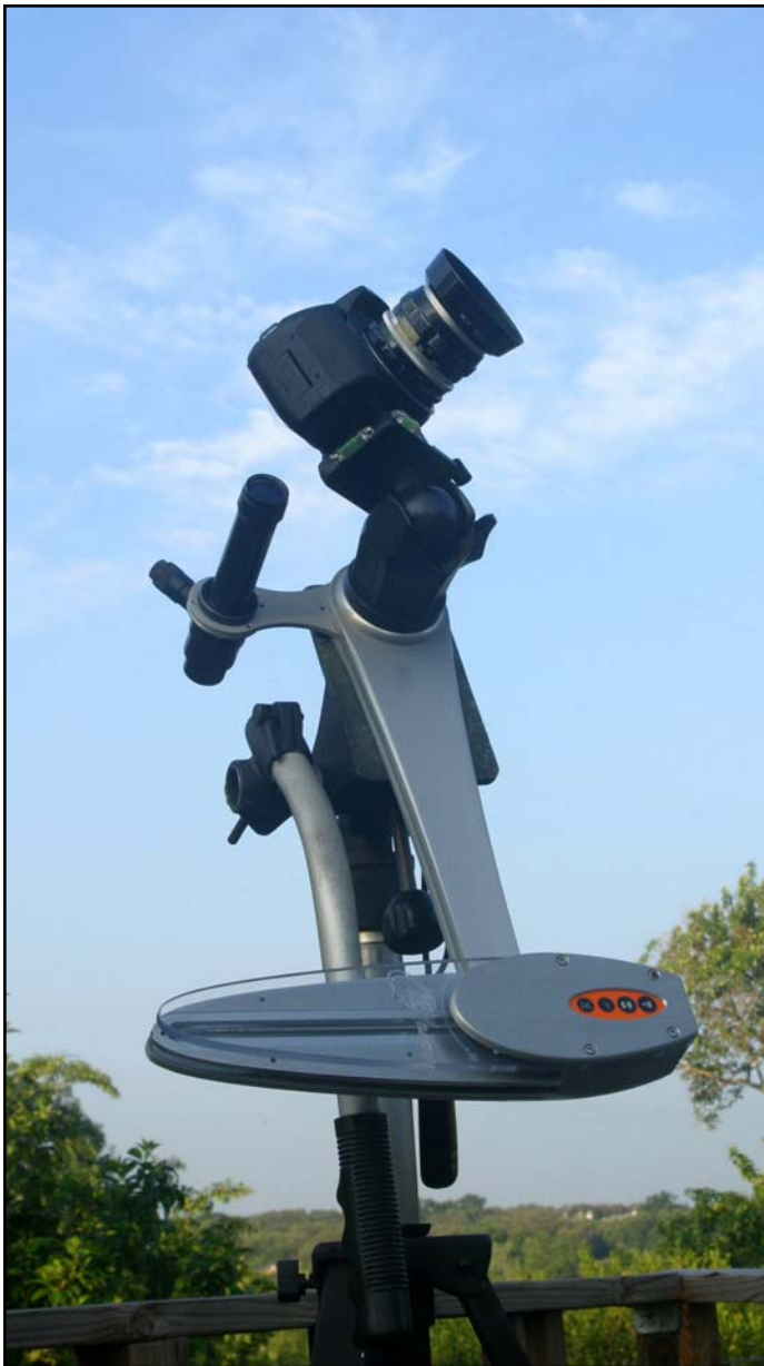
The AstroTrac is attached to a tripod and the drive screw assembly is rotated to the left for northern hemisphere use
