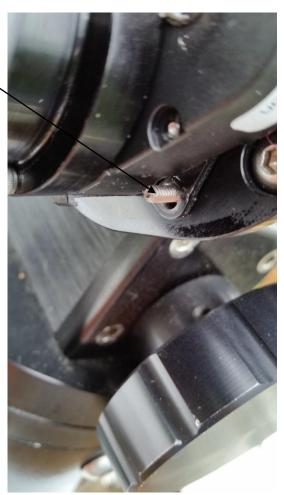
A simple solution: wind some brass shim around the bolt. In place, the shims keep the gearbox from shifting.
