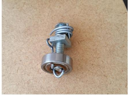
Insert the 2 wire jaws into the bearing center hole, and then screw in the bolt to keep the 2 jaws from retracting back out of the hole. Pull the bearing out. The picture above shows the bearing puller, and the bearing still in the jaws of the wire puller.
