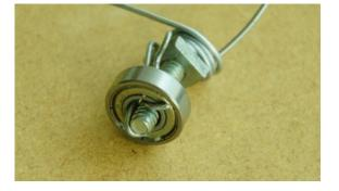
Post-script Aug 7 2016: Two owners found that this simple puller was not able to remove the bearing, and they resorted to drilling out the end of the right bearing block with a small hole, and then pushed out the bearing from there. I then made a similar puller to the one above by bending some steel nails into thicker jaws, and hooking those above the bearing with steel wire. I have sent this to Masami Yamada in Tokyo to try.
