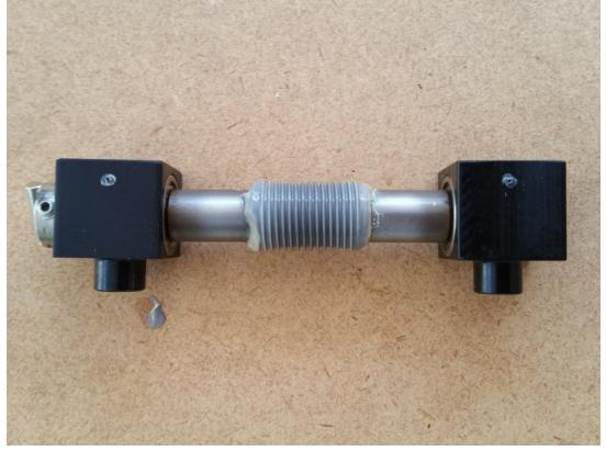
Pull the worm out of the right hand (rear) bearing block.
