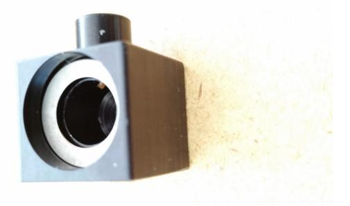
Now use some 2000 grit or similar very fine grit sandpaper to polish down the outer diameter of the bearing, and put some lubricant (I used SS2000 teflon grease) around the bearing so it will slide on the sides of the block hole. I was careful to NOT overpolish the inside of the block, or outside of the bearing, to cause the bearing to have play perpendicular to the worm axis.
