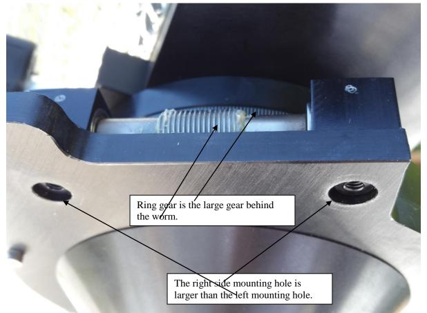
Now complete bolting in the left underneath bolt until snug, and snug the right underneath bolt. This right side bolt position must be adjusted so that the worm is not too tight against the larger ring gear teeth.
