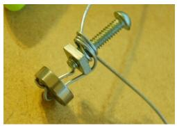
Step 6: pull out the bearing from the block.
