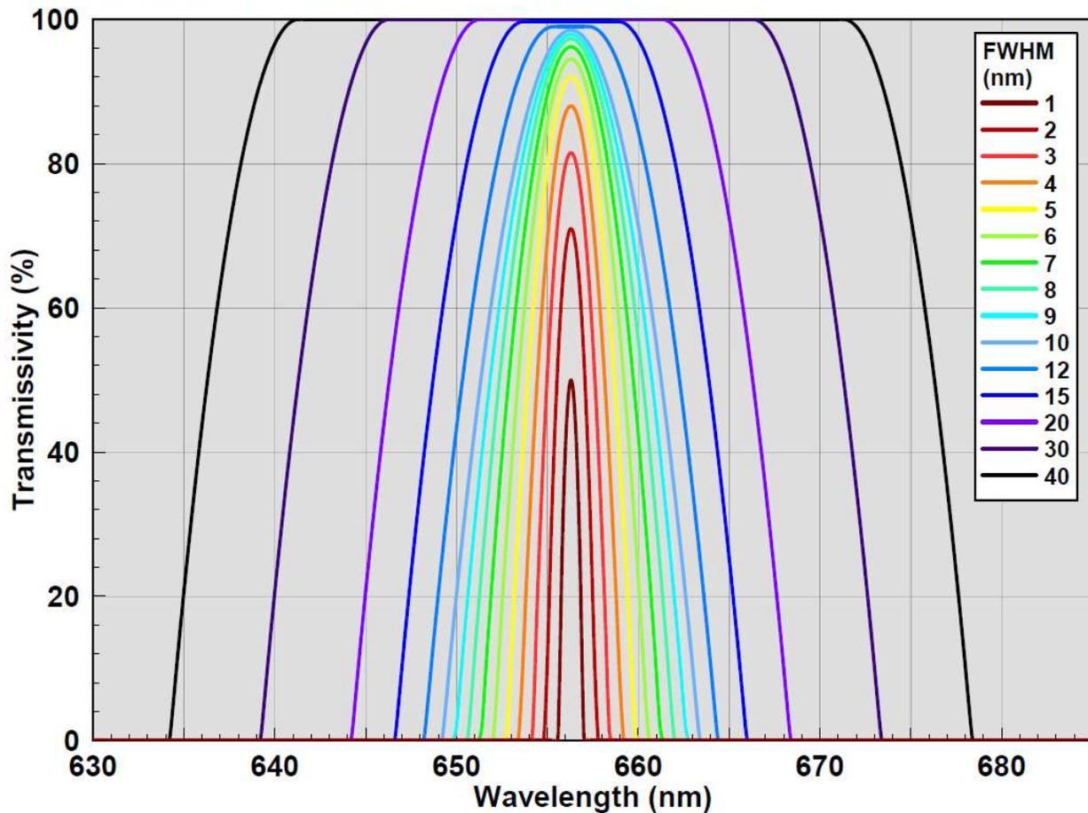
Figure 1 Spectral Response of Generic H-alpha Narrowband Filters
