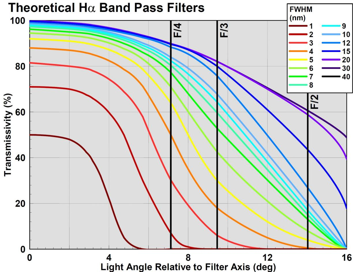
Figure 4 Predicted Generic Filter H-alpha Transmission vs Angle
