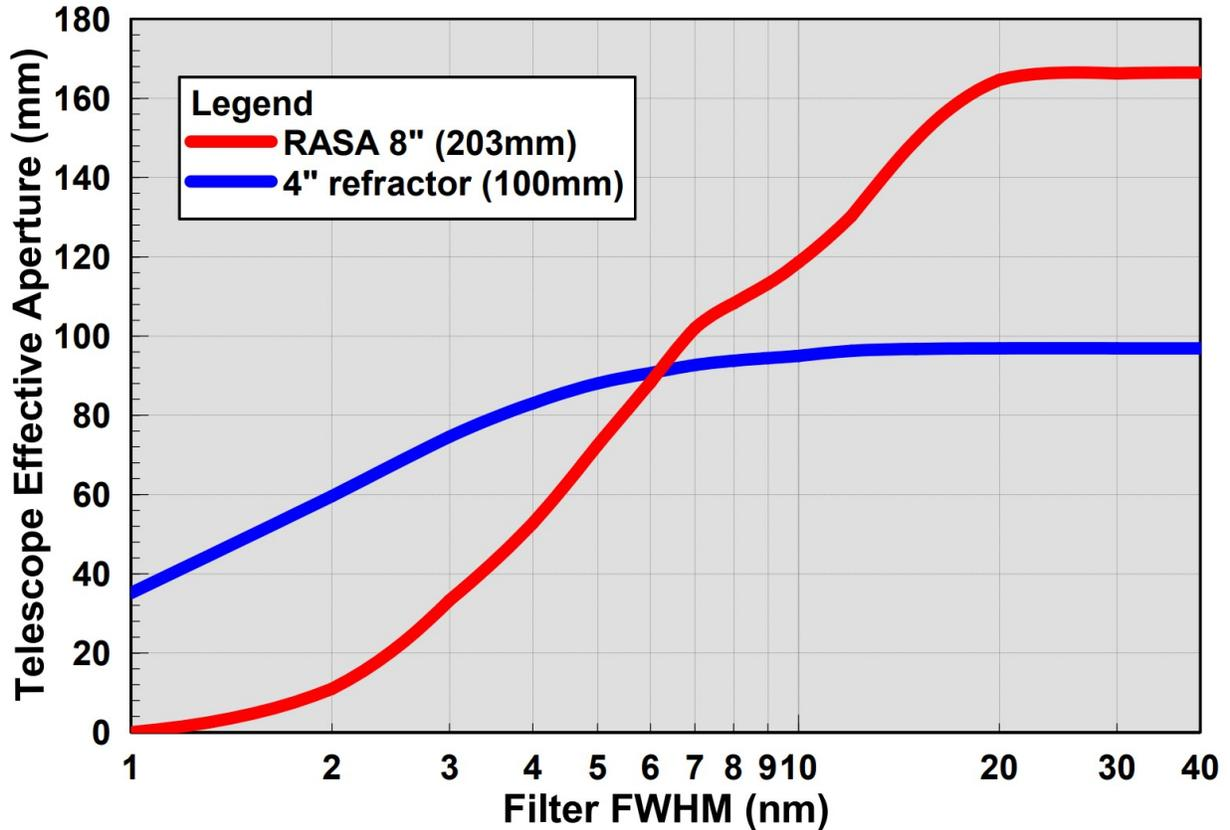
Figure 5 Predicted Scope Effective Aperture vs Filter FWHM
