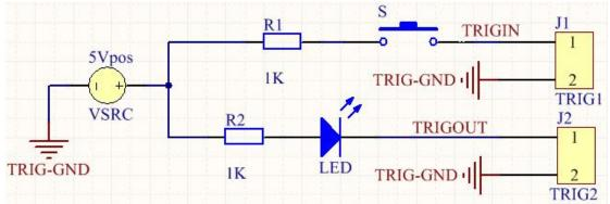
About the camera TRIG module work principle, please refer to the follow circuit:
