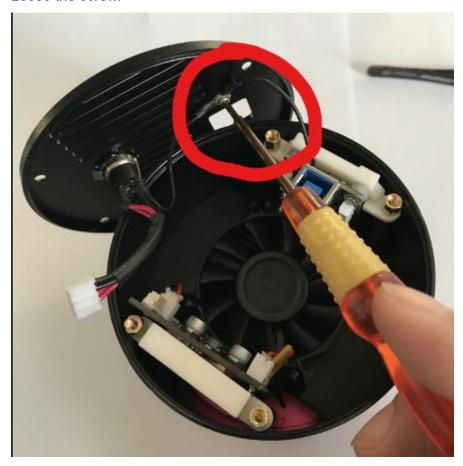
4. Remove the camera shell and reconnect the brown flat cable
