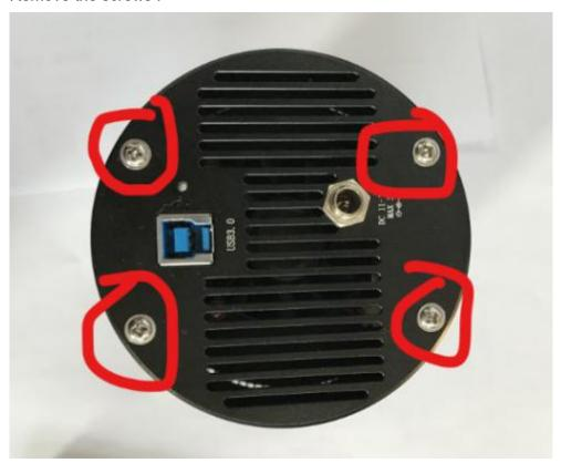
2. Open the bottom cover of the camera, disconnect the power connector with tweezers.
