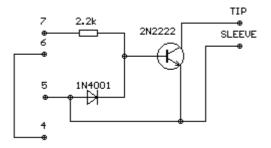
Numbers on the scheme are numbers of RS-232 pins. The idea of this circuit is to make a connection between TIP and SLEEVE when pin7 (RTS) is high (positive voltage), and to disconnect them when RTS is low (negative voltage). Voltage on the transistor base should be approximately 0.7V. Diode in this circuit only protects the transistor and does not play any other role. Not bad idea is to place the whole circuit in the DB-9 plug.
