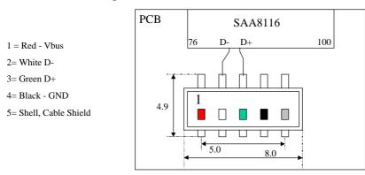
To be connected to USB cable with female adapter on one side and USB A plug (rectangular one) on the other side.
