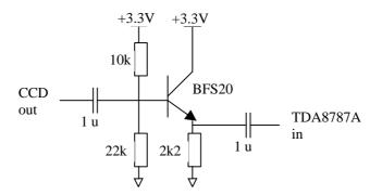
In the case of the Sony ICX098 CCD, the CCD already contains a buffer. The outside buffer can then be removed. Then care must be taken during the camera alignment procedure, that the CCD output never exceeds the maximum amplitude of the TDA8787A input. This is done by setting the nominal AGC value.
