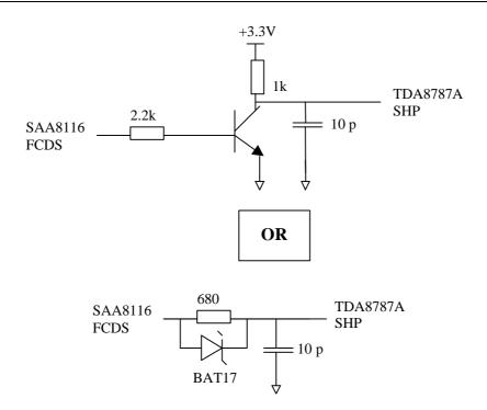
On this last schematic, a BAT17 can be used because it has a low forward voltage and a low parasitic capacitance. This solution results in a about 15 ns SHP pulse width. A standard diode BAS16 could also be chosen as a cheapest solution, although it gives less good results (about 12 ns SHP pulse width).
