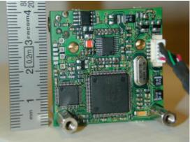
The goal of this reference design is to demonstrate the functionality and the performances of the SAA8116 in a CCD application.
